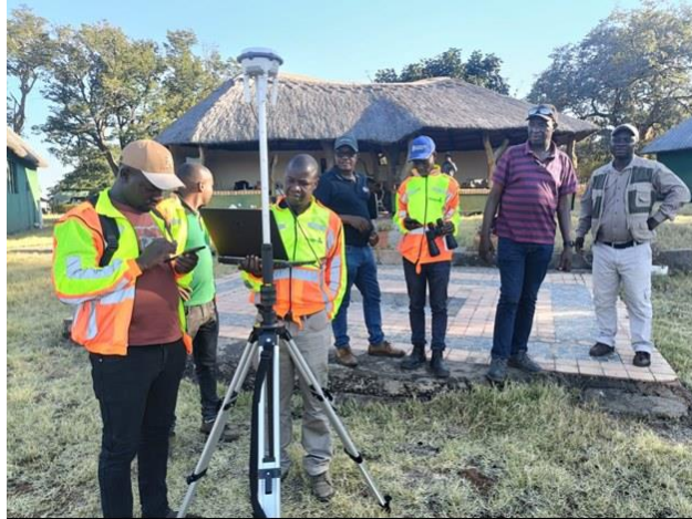
8 - Calibration of RTK device to improve coordinates accuracy
